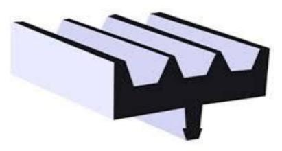
Material : EPDM100x85x20mmMass : 150-165 gms ApproximatelyHardness : 80±5 IRHD (International Rubber Degree of Hardness)
